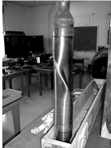
Figure III-9-12. Torsion failures. Helicopter turbine (left); Turbine engine shaft failure (right)
