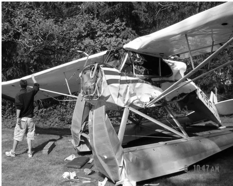
Figure III-5-1. Water impact damage
