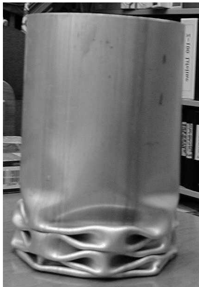
Figure III-9-9. Compression (buckling) failure (left); Block compression failure (right)
