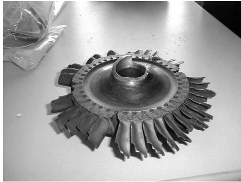
Figure III-9-12. Torsion failures. Helicopter turbine (left); Turbine engine shaft failure (right)
