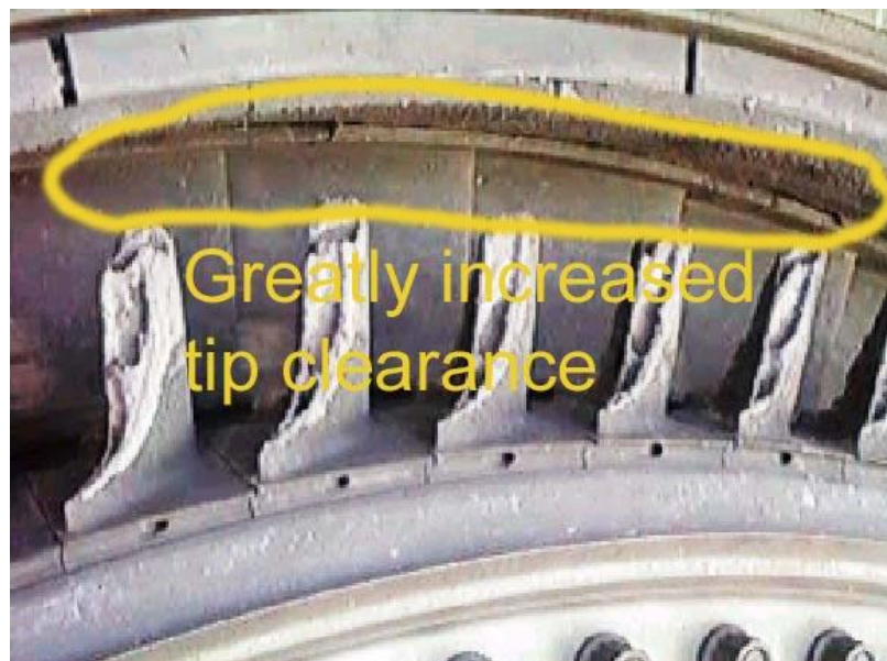
Figure III-12-24. Increased tip clearance caused by overheating
