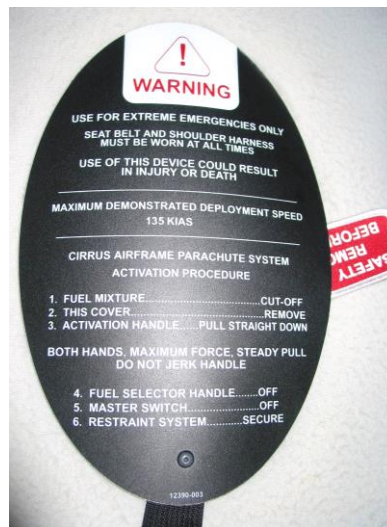
Figure III-13-12. Roof mounted CAPS activation handle cover
