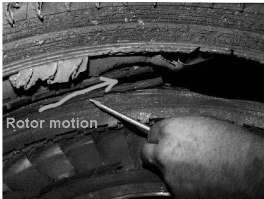
Figure III-12-13. Squeeze-rupture penetration hole
