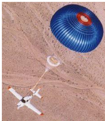
Figure III-13-11. Rocket-deployed emergency parachute system
