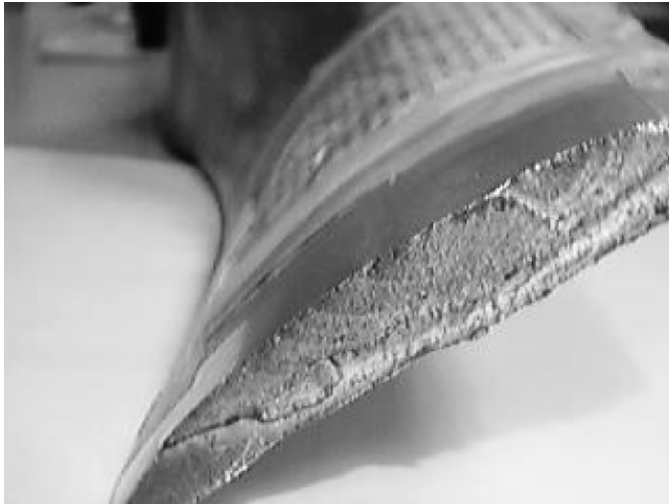
Figure III-12-37. Propeller showing beach rings as a result of resonance fatigue failure
